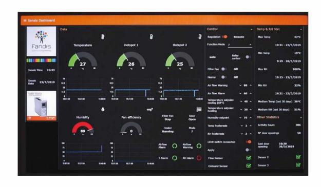
Pre-configures dashboard that allows to monitor the main values, fix setpoints and other setup data in local mode before the device is connected to the network or to another master unit
