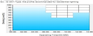
Set up for D01-Type in Smart timer dimming software program:
