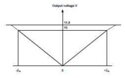
Note: 1) The performance specified in the datasheet is valid within the 0-10 V DC output range only.
