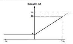
Note: 17 The performance specified in the datasheet is valid within the 4-20 mA output range only.
