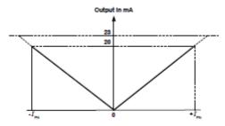
Note: 1) The performance specified in the datasheet is valid within the 0-20 mA output range only.
