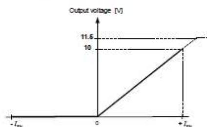
Note: <sup>1)</sup> The performance specified in the datasheet is valid within the 0-10 V output range only.
