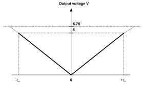
Note: 1) The performance specified in the datasheet is valid within the 0-5 V DC output range only.
