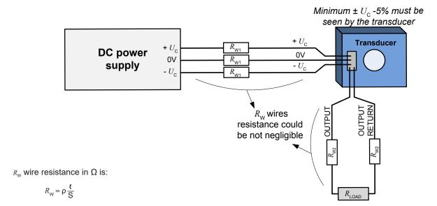
S: Cross section of wire in m<sup>2</sup>
