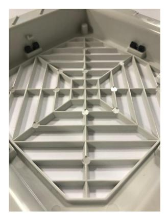
6) The lower part of the **cover** has two openings that, combined with the slight inclination of the interior part of the base, facilitate the water runoff to the outside and limit the water accumulation in the filter.
