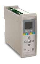
Sensis is a smart Thermal Management device for enclosure that meets alone all the needs of climate control, predictive maintenance and inter-connectivity. Sensis measures the temperature and humidity inside the enclosure, registers the exceeding of critical thresholds or the opening of cabinet door, as well as interacts with the main field buses or the network.
