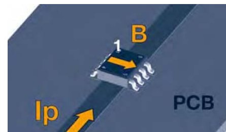
Fig. 2: One possible PCB design; The track is located underneath the Minisens
