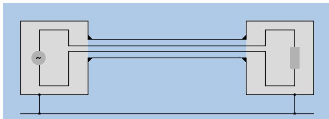
Proper connection of shielded cable ends
