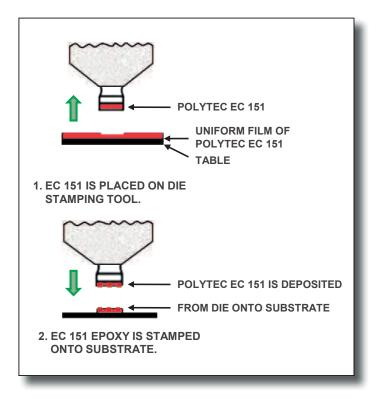
(75  $\mu$ m thickness) is transferred to the substrate – the rest remains on the stamp.
