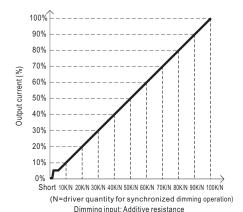
Note: 1. Min. dimming level is about 8% and the output current is not defined when 0% < Iout < 8%.
