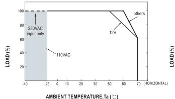
$\bigcirc$  If ELG-200 operates in Constant Current mode with the rated current, the maximum workable Ta is 50  $^{\circ}\mathbb{C}$  for 12V-model whereas 60  $^{\circ}\mathbb{C}$  for other models.
