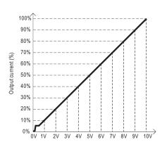
Dimming input: Additive voltage
