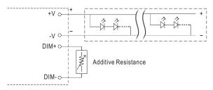
"DO NOT connect "DIM- to -V"
