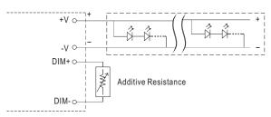
"DO NOT connect "DIM- to -V"
