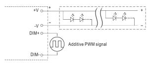
"DO NOT connect "DIM- to -V"
