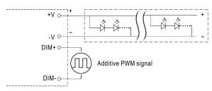
"DO NOT connect "DIM- to -V"
