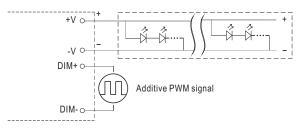
"DO NOT connect "DIM- to -V"
