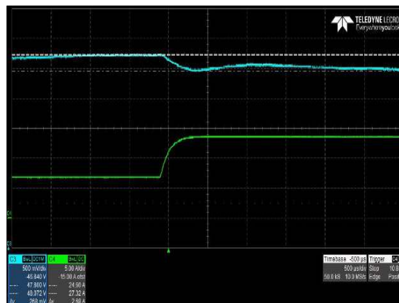
Figure 31: CNS658-MU Transient Response – V_o Deviation (Low to High) V_{IN} = 90\text{Vac} , I_o = 50\% to 100% load, Output Cap = 330 \mu\text{F} /A Ch 3: V_o Ch 4: I_o
