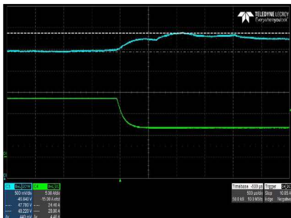
Figure 30: CNS658-MU Transient Response – V_o Deviation (High to Low) V_{IN} = 90\text{Vac} , I_o = 100\% to 50% load, Output Cap = 330 \mu\text{F} /A Ch 3: V_o Ch 4: I_o
