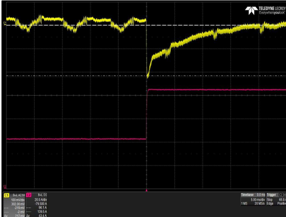
Figure 7: LCM1000L-T Transient Response - Vo Deviation 50% to 100% load change 1A/uS slew rate Vin = 90Vac Ch 1: Vo Ch 2: Io
