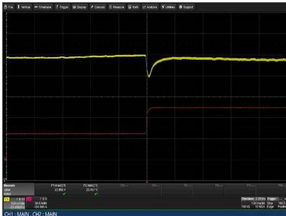
Figure 23: LCM3000Q-T Transient Response - Vo Deviation 50% to 100% load change 1A/uS slew rate Vin = 230Vac Ch 1: Vo Ch 2: Io
