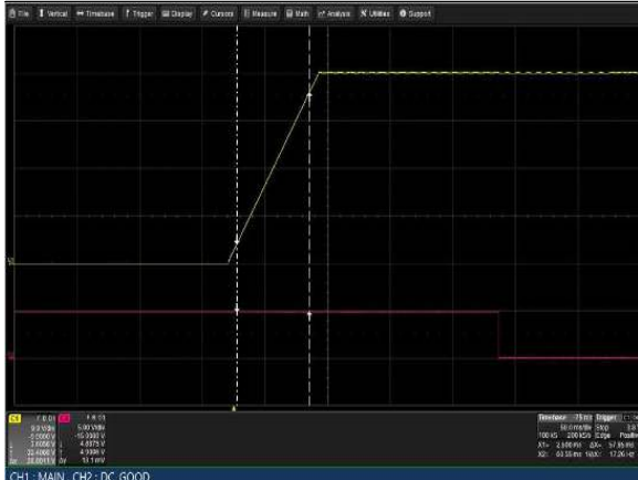
Figure 35: LCM3000U-T Output Voltage Startup V_{in} = 264V_{ac} Load: I_o = 83.3A (36V), I_{sb} = 2A Ch 1: Vo Ch 2: G_DCOK_C
