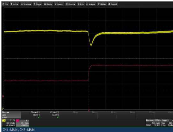
Figure 51: LCM3000W-T Transient Response - Vo Deviation 50% to 100% load change 1A/uS slew rate V_{in} = 230V_{ac} Ch 1: Vo Ch 2: Io
