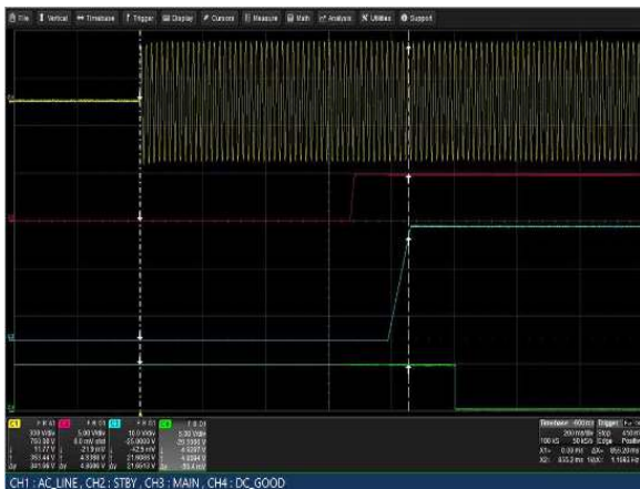
Figure 17: LCM3000Q-T Turn-on delay via AC mains
