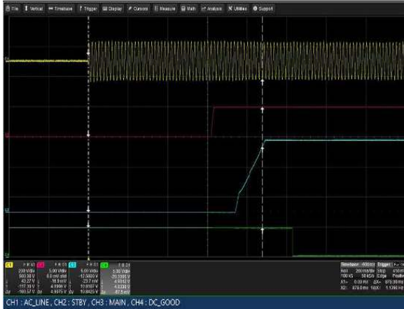
Figure 1: LCM3000L-T Turn-on delay via AC mains
