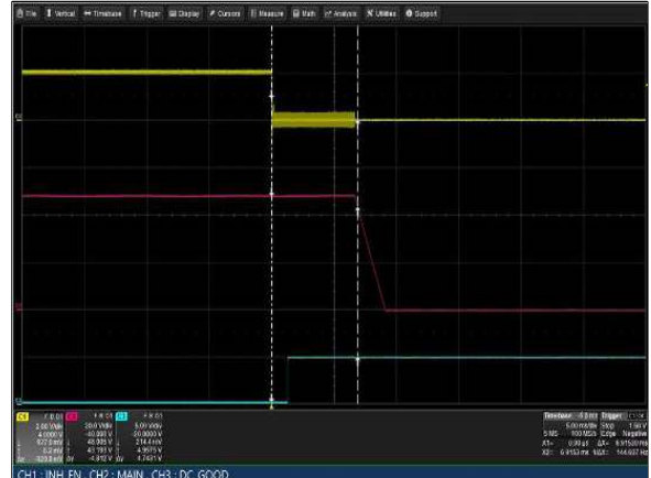
Figure 50: LCM3000W-T Turn Off Characteristic via INH_EN V_{in} = 264V_{ac} Load: I_o = 62.5A (48V), I_{sb} = 2A Ch 1: INH_EN Ch 2: Vo Ch 3: G_DCOK_C
