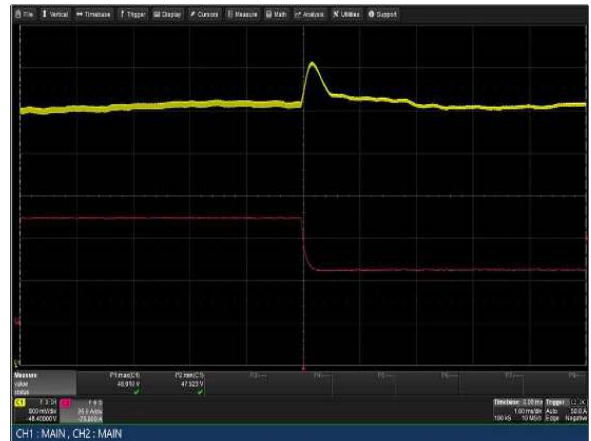
Figure 52: LCM3000W-T Transient Response - Vo Deviation 100% to 50% load change 1A/uS slew rate V_{in} = 230V_{ac} Ch 1: Vo Ch 2: Io
