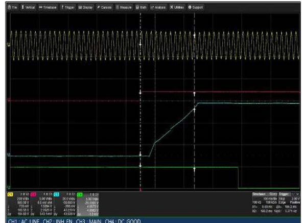
Figure 44: LCM3000W-T Turn-on delay via INH_EN
