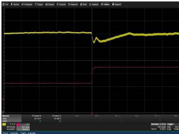
Figure 37: LCM3000U-T Transient Response - Vo Deviation 50% to 100% load change 1A/uS slew rate V_{in} = 230V_{ac} Ch 1: Vo Ch 2: Io
