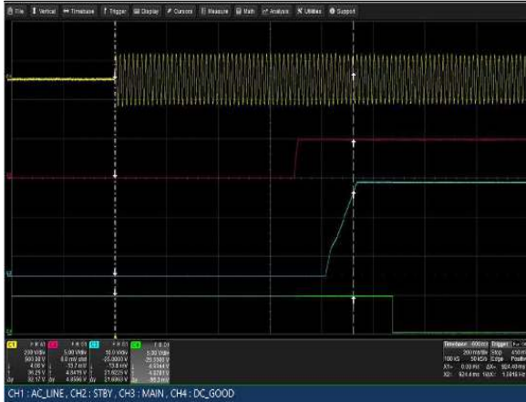
Figure 15: LCM3000Q-T Turn-on delay via AC mains
