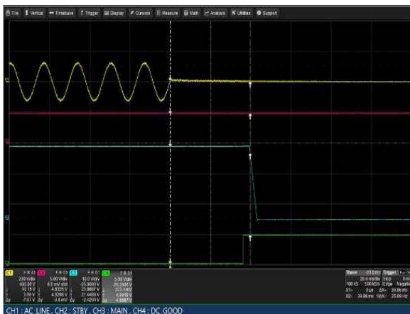
Figure 19: LCM3000Q-T Hold-up Time
