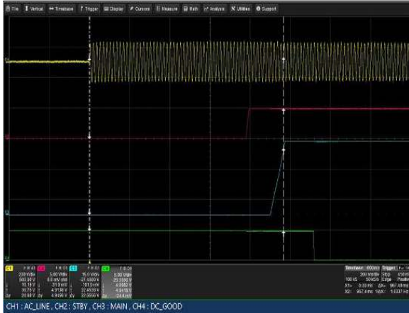
Figure 29: LCM3000U-T Turn-on delay via AC mains
