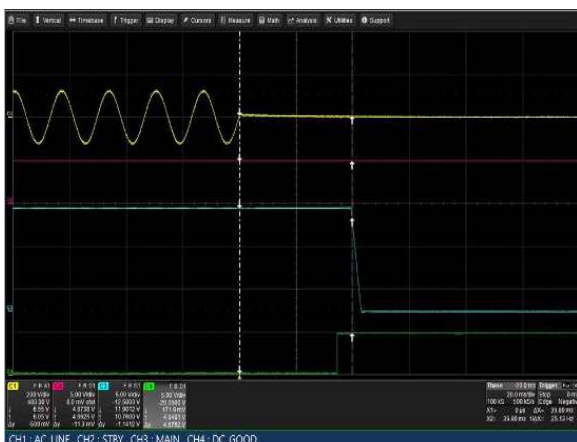
Figure 5: LCM3000L-T Hold-up Time
