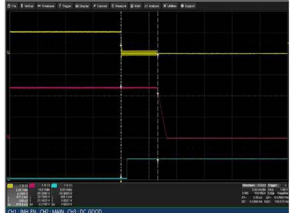
Figure 22: LCM3000Q-T Turn Off Characteristic via INH_EN Vin = 264Vac Load: Io = 125A (24V), Isb = 2A Ch 1: INH_EN Ch 2: Vo Ch 3: G_DCOK_C
