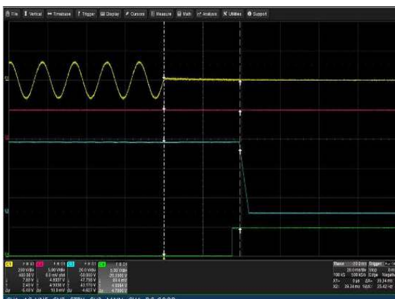
Figure 47: LCM3000W-T Hold-up Time
