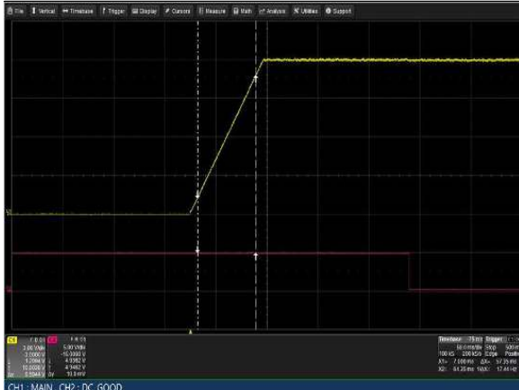
Figure 7: LCM3000L-T Output Voltage Startup V_{in} = 264V_{ac} Load: I_o = 125A ( 12V ), I_{sb} = 2A Ch 1: Vo Ch 2: G_DCOK_C
