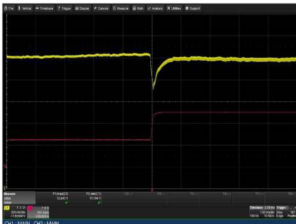
Figure 9: LCM3000L-T Transient Response - Vo Deviation 50% to 100% load change 1A/uS slew rate V_{in} = 230V_{ac} Ch 1: Vo Ch 2: I_o
