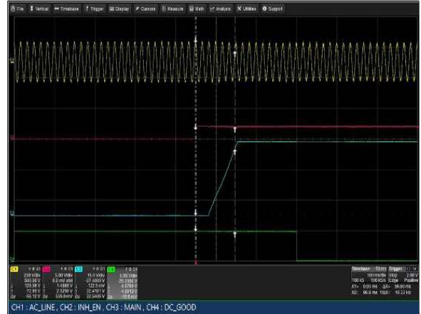
Figure 30: LCM3000U-T Turn-on delay via INH_EN
