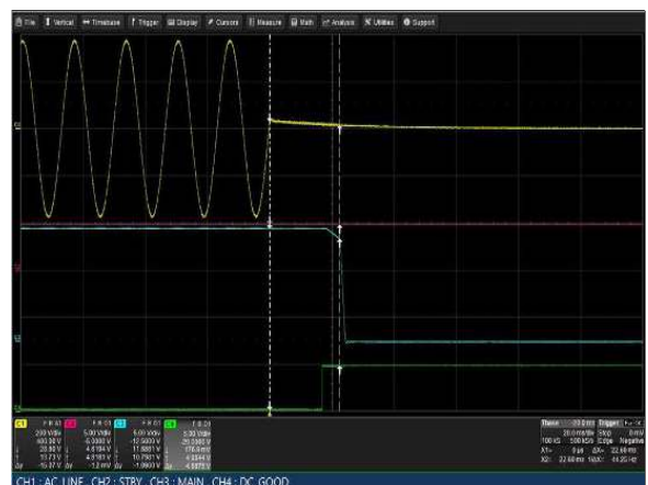
Figure 6: LCM3000L-T Hold-up Time
