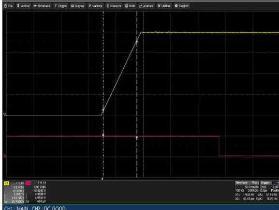
Figure 21: LCM3000Q-T Output Voltage Startup Vin = 264Vac Load: Io = 125A (24V), Isb = 2A Ch 1: Vo Ch 2: G_DCOK_C
