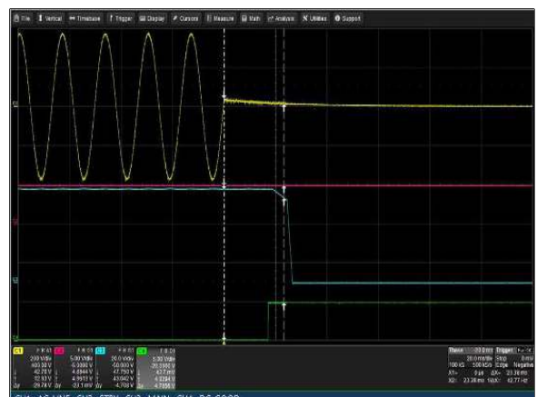
Figure 48: LCM3000W-T Hold-up Time
