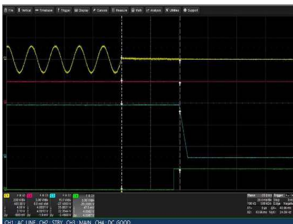
Figure 33: LCM3000U-T Hold-up Time
