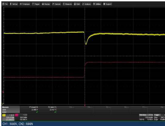
Figure 23: LCM3000Q-T Transient Response - Vo Deviation 50% to 100% load change 1A/uS slew rate V_{in} = 230V_{ac} Ch 1: Vo Ch 2: Io
