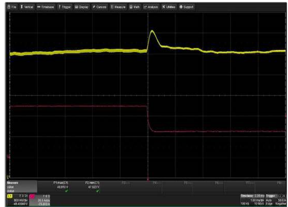
Figure 52: LCM3000W-T Transient Response - Vo Deviation 100% to 50% load change 1A/uS slew rate V_{in} = 230V_{ac} Ch 1: Vo Ch 2: Io
