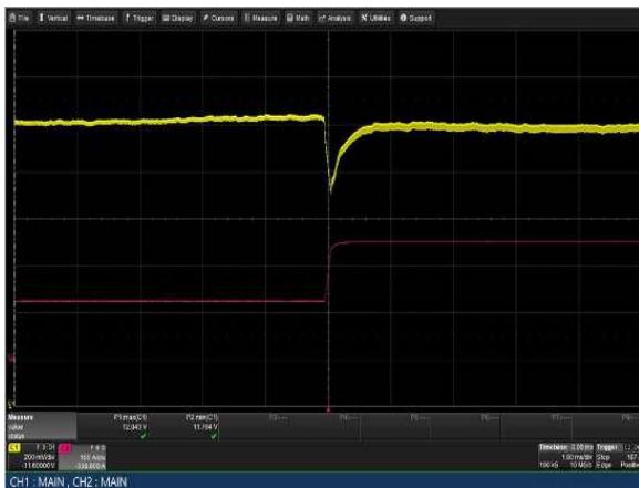
Figure 9: LCM3000L-T Transient Response - Vo Deviation 50% to 100% load change 1A/uS slew rate V_{in} = 230V_{ac} Ch 1: Vo Ch 2: I_o
