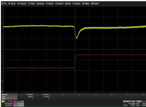
Figure 51: LCM3000W-T Transient Response - Vo Deviation 50% to 100% load change 1A/uS slew rate V_{in} = 230V_{ac} Ch 1: Vo Ch 2: Io
