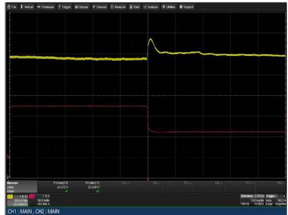
Figure 24: LCM3000Q-T Transient Response - Vo Deviation 100% to 50% load change 1A/uS slew rate V_{in} = 230V_{ac} Ch 1: Vo Ch 2: Io
