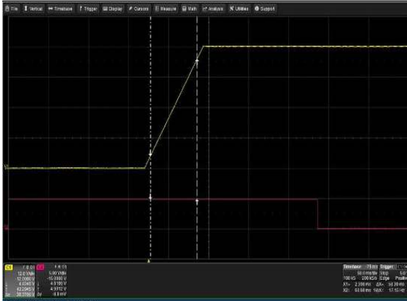
Figure 49: LCM3000W-T Output Voltage Startup V_{in} = 264V_{ac} Load: I_o = 62.5A (48V), I_{sb} = 2A Ch 1: Vo Ch 2: G_DCOK_C
