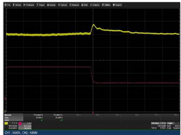
Figure 38: LCM3000U-T Transient Response - V_o Deviation 100% to 50% load change 1A/uS slew rate V_{in} = 230V_{ac} Ch 1: V_o Ch 2: I_o
