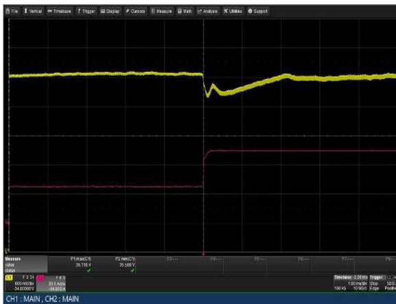
Figure 37: LCM3000U-T Transient Response - V_o Deviation 50% to 100% load change 1A/uS slew rate V_{in} = 230V_{ac} Ch 1: V_o Ch 2: I_o
