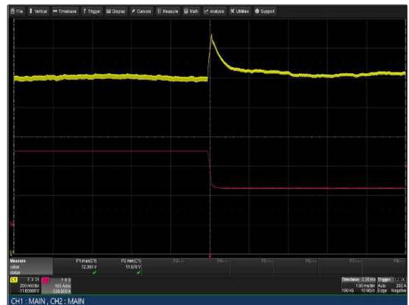
Figure 10: LCM3000L-T Transient Response - Vo Deviation 100% to 50% load change 1A/uS slew rate V_{in} = 230V_{ac} Ch 1: Vo Ch 2: I_o
