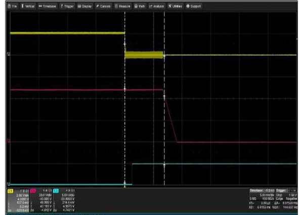
Figure 50: LCM3000W-T Turn Off Characteristic via INH_EN V_{in} = 264V_{ac} Load: I_o = 62.5A (48V), I_{sb} = 2A Ch 1: INH_EN Ch 2: Vo Ch 3: G_DCOK_C
