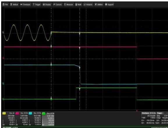
Figure 14: LCM600N Hold-up Time Vin = 90Vac / 63Hz / 0° Load: Io = 40A (15V), I SB = 2A (5V) Ch 1: AC Mains Ch 2: V SB Ch 3: V o Ch 4: G_DCOK_C
