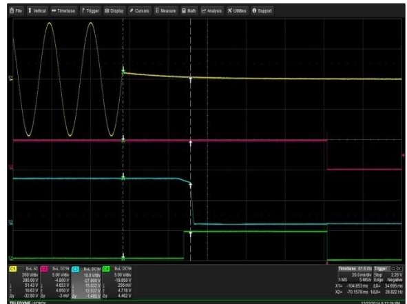
Figure 15: LCM600N Hold-up Time Vin = 264Vac / 47Hz / 0° Load: Io = 40A (15V), I SB = 2A (5V) Ch 1: AC Mains Ch 2: V SB Ch 3: V o Ch 4: G_DCOK_C
