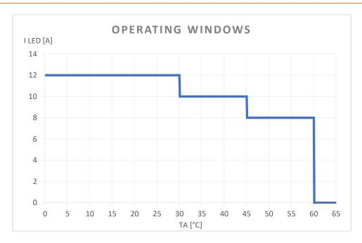
Below are the maximum current values that can be supplied by the MINI-1CV device when the working temperature varies. Ambient temperature [Ta]:
