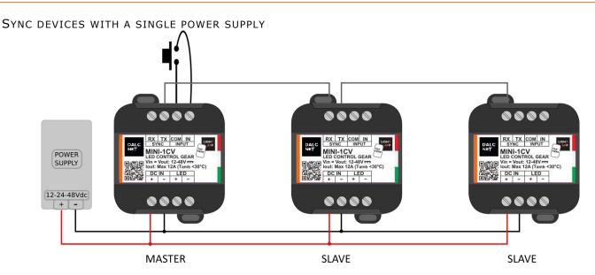
DEVICE SYNCHRONIZATION, A DIMMER POWER SUPPLY
