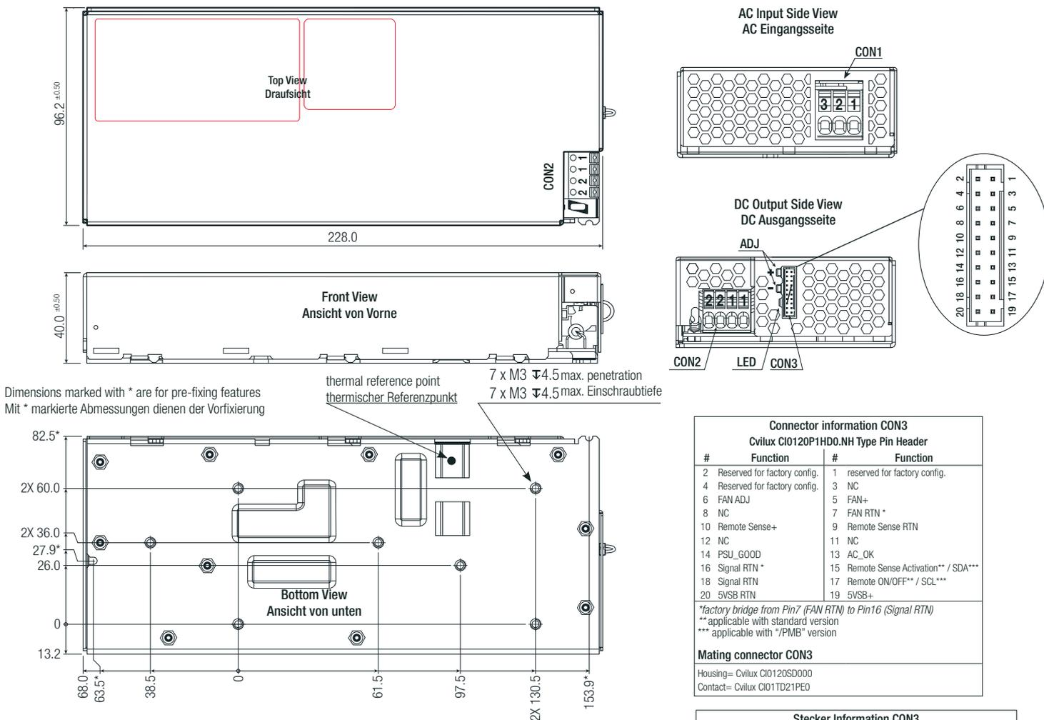
Dimensions marked with \* are for pre-fixing features
