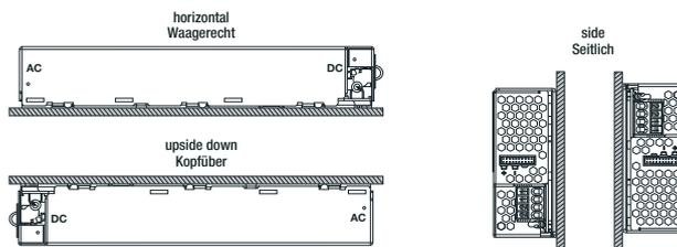
Recommended orientation horizontal side or upside down: no derating is required.
