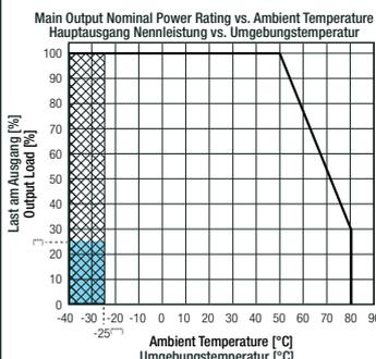
\*\*\*Output Power at T<sub>amb</sub> = -40°C cold start ≤250W.
