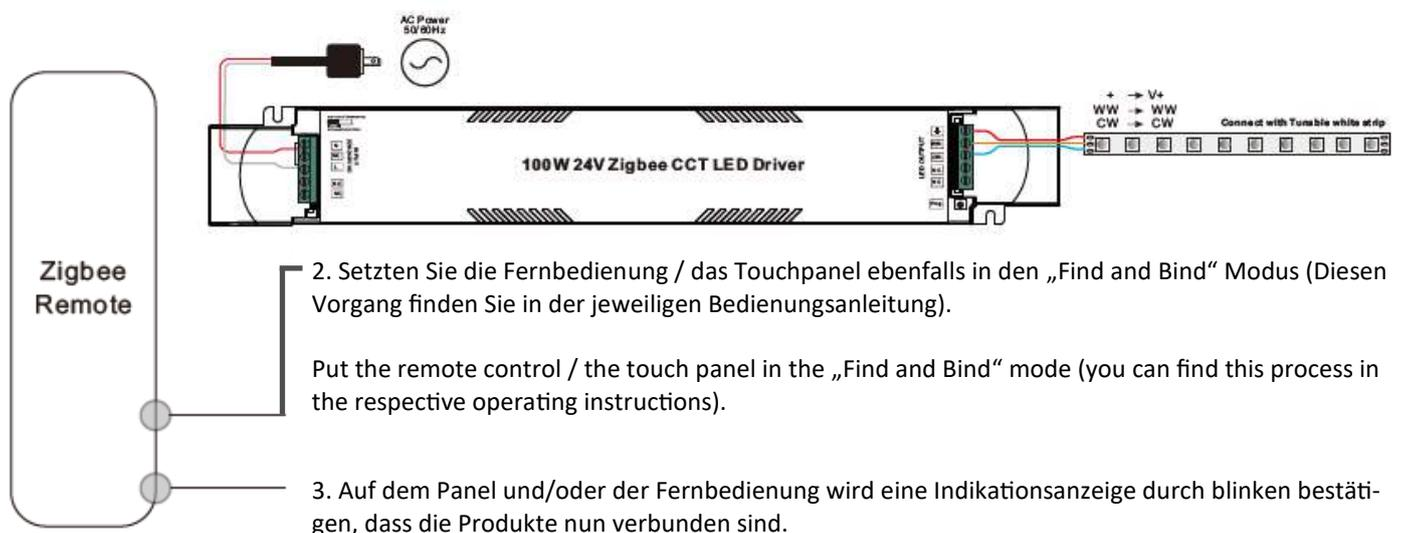
An indicator on the panel and/or remote control will flash to confirm that the products are now connected.
