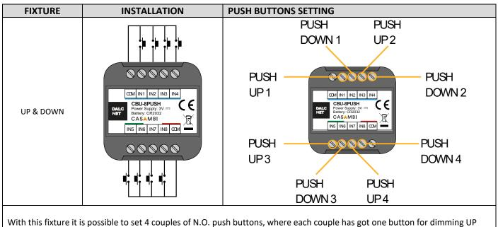
luminaire and one for dimming Down. In total there can be connected 8 N.O. push buttons.
