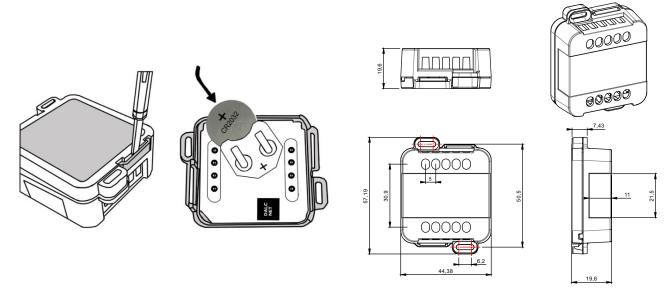
Note: The inserted battery of type CR 2032 can last from 2-5 years.
