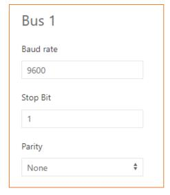
The fields displayed in the MODBUS RTU Slave section for Bus 1 (or Bus 2) are:
