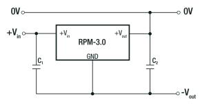
${\bf C_1}$  and  ${\bf C_2}$  may be added to reduced ripple and should be fitted close to the converter pins.
