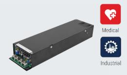
Advanced Energy's SL Power NGB1200 medically-approved AC-DC power supplies are available with a nominal main output of 12 V, 15 V, 24 V or 48 V. Auxiliary 5 V output is also provided. NGB1200 power supplies provide 1200 Watts of output power. All models have output overvoltage, short circuit and overload protection and a 3 x 10.5 x 1.6 inch form factor with built-in fan.
