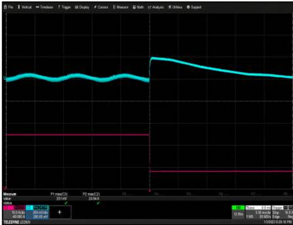
Figure 18: NGB800S24K Transient Response - Vo Deviation Vin = 115Vac Load: Io = 75% to 25%, 0.2A/μs slew rate Ch 2: Io Ch 3: Vo
