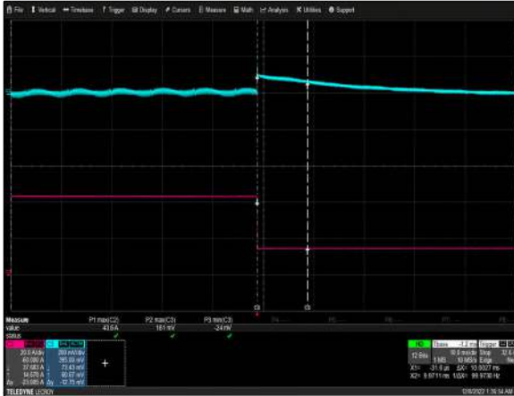
Figure 7: NGB800S12K Transient Response - V_o Deviation V_{in} = 115V_{ac} Load: I_o = 75\% to 25\% , 0.2A/\mu s slew rate Ch 2: I_o Ch 3: V_o
