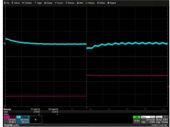
Figure 30: NGB800S48K Transient Response - V_o Deviation V_{in} = 115V_{ac} Load: I_o = 25\% to 75\% , 0.2A/\mu s slew rate Ch 2: I_o Ch 3: V_o
