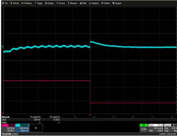
Figure 29: NGB800S48K Transient Response - V_o Deviation V_{in} = 115V_{ac} Load: I_o = 75\% to 25\% , 0.2A/\mu s slew rate Ch 2: I_o Ch 3: V_o
