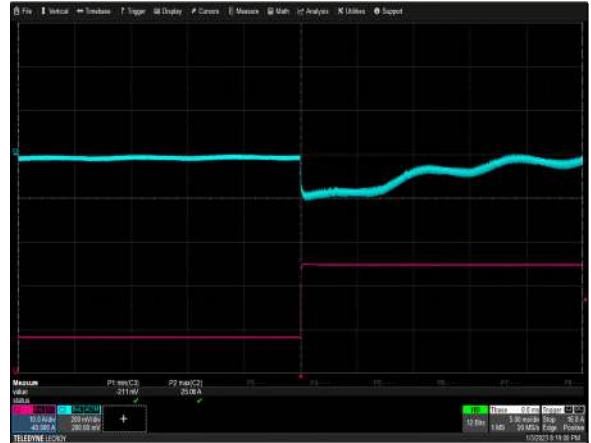
Figure 19: NGB800S24K Transient Response - Vo Deviation Vin = 115Vac Load: Io = 25% to 75%, 0.2A/μs slew rate Ch 2: Io Ch 3: Vo
