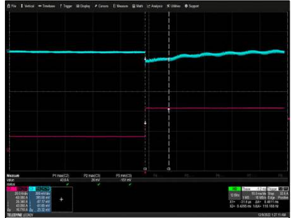
Figure 8: NGB800S12K Transient Response - V_o Deviation V_{in} = 115V_{ac} Load: I_o = 25\% to 75\% , 0.2A/\mu s slew rate Ch 2: I_o Ch 3: V_o
