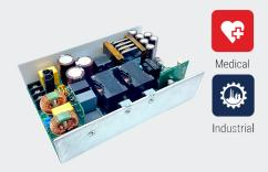
Advanced Energy's SL Power NGB660 medically-approved AC-DC power supplies are available with a nominal main output of 12 V, 15 V, 24 V, or 48 V. NGB660 power supplies provide up to 660 Watts of output power with air flow. All models have output overvoltage, short circuit and overload protection and a 4 x 6 x 1.6 inch form factor.
