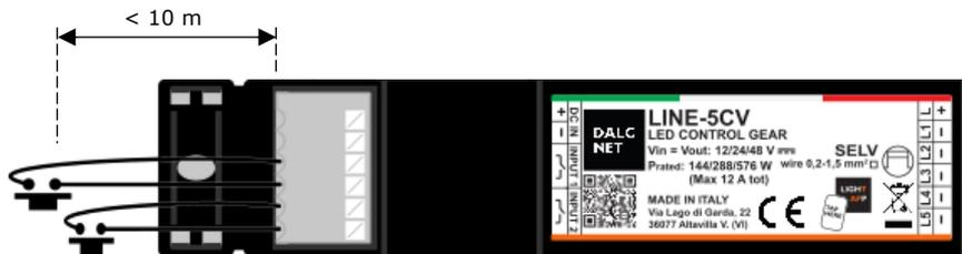
Figure 7: Local Command connection diagram for Short Distances
