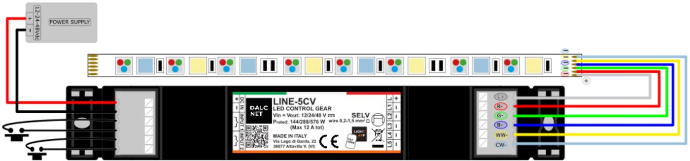
Figure 6: Connection diagram for RGB+TW LED load
