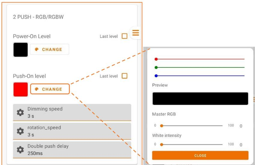
**Power-On Level:** Sets the RGB and white light levels to which the output is brought as soon as the device is powered. The RGB and intensity parameters can be set via the "Change" submenu.
