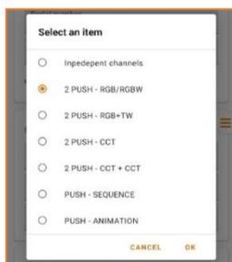
Within the "Control Type" configuration it is possible to select from 7 types of controls available for LINE-5CV
