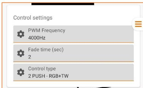
On the *Control Settings* screen, you can configure the different parameters for the driver's operation mode.
