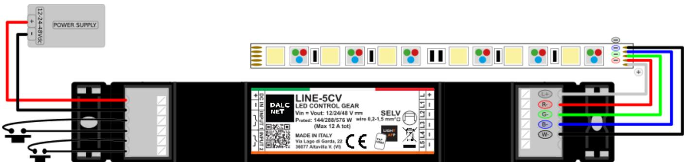
Figure 5: Connection diagram for RGBW LED load
