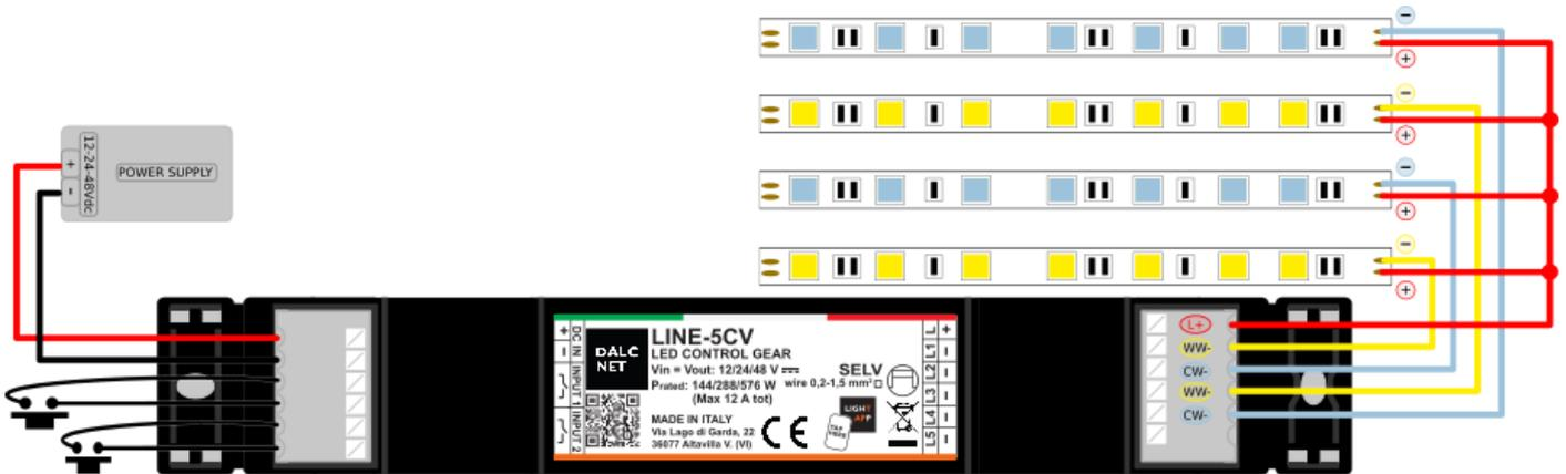
Figure 3: Connection diagram for Tunable White LED loads
