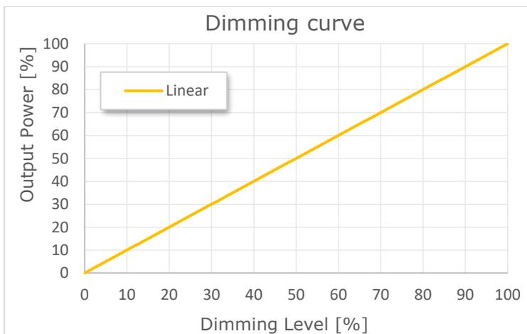
Figure 12: Dimming Curve
