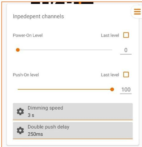
**Power-On Level:** this is the intensity value to which the output is brought as soon as the device is powered.
