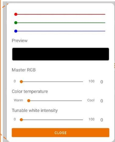
**Power-On Level:** Sets the RGB and white light levels to which the output is brought as soon as the device is powered. The RGB and intensity parameters can be set via the "Change" submenu.
