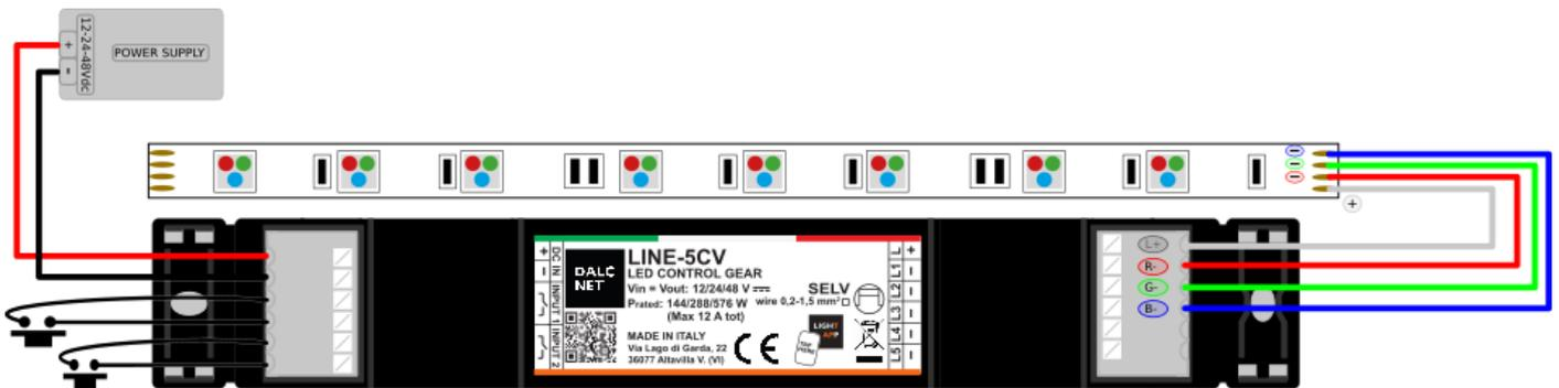
Figure 4: Connection diagram for RGB load
