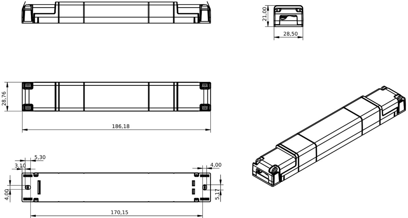
Figure 13: Mechanical dimensions
