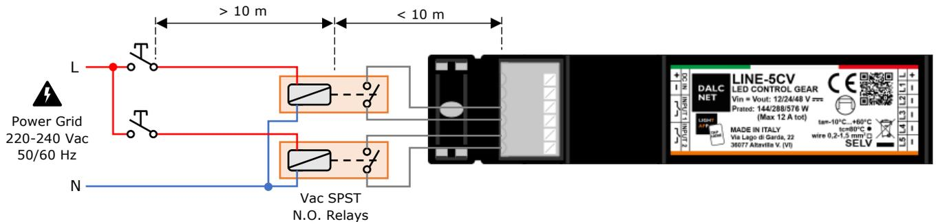
Figure 8: Local Command connection diagram for Long Distances
